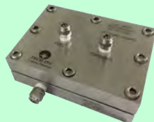
Reverse Osmosis Test Cell
