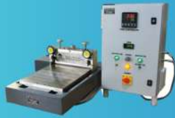
FLATSHEET MEMBRANE CASTING MACHINE WITH HEATING FACILITY
